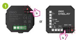
To properly link thermostat with the module/relay first click quickly the button on the device 5 times. The LED diode will start flashing slowly on red, which means the device is in binding mode.
